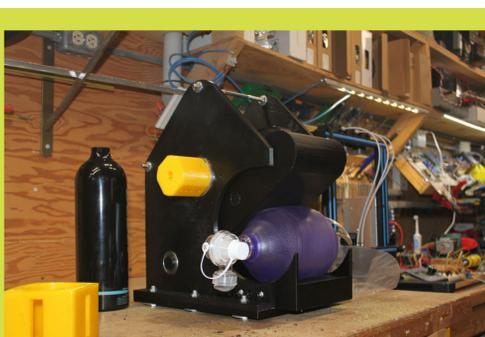
In line with the College's vision to transform lives and communities, the Wearable, Interactive and Mobile Technology Access Center in Health (WIMTACH) is working virtually to develop a novel, portable ventilator to assist with respiratory care for COVID-19 patients. This idea and design have been developed by WIMTACH team members Dr. Yashodhan Athavale, Dr. Pouria Tavakkoli, Zeziel Vidad, Majura Maheswaran, Director of WIMTACH Dr. Purnima Tyagi, and SETAS Professor Robert Wickson.
